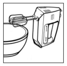
the bowl when using a handheld utensil, move the Speed Control to the Off position and place the Mixer on its Heel Rest so the Beaters can drain into the bowl. (Figure B)
